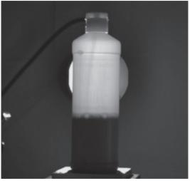
Detect & Control solid filling level inside a plastic container
